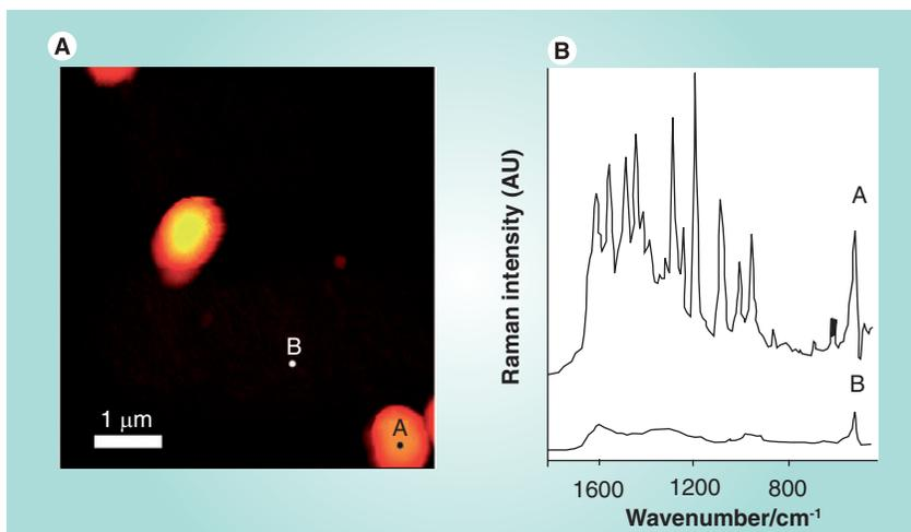
**Figure 3. An example of tip-enhanced Raman spectroscopy of bacterial cells.** Topographic image of *Staphylococcus epidermidis* cells (A) with the positions marked from where Raman spectra (B) were measured. Position A corresponds to a tip-enhanced Raman spectroscopy spectrum on the cell surface, and position B corresponds to a reference tip-enhanced Raman spectroscopy experiment on the glass surface. Reproduced with permission from [36] © Wiley-VCH Verlag GmbH & Co. KGaA.
