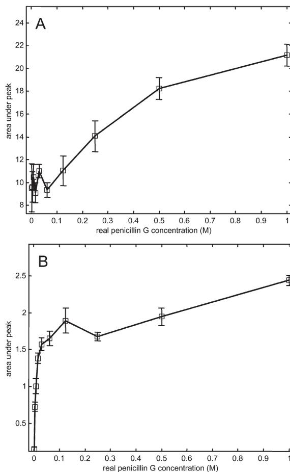
**Fig. 5** Plots of the peak areas for Raman (A) and SERS (B) of the benzene ring at 1005 cm<sup>-1</sup> versus the penicillin G concentration. (A) Peak areas from Raman spectra show that 0.05–1 M penicillin G is quantifiable. (B) Peak areas from SERS spectra showing that below 0.1 M penicillin G the SERS response is quantifiable: by contrast above 0.2 M penicillin G a quantifiable Raman response is seen. Data plotted as means with standard deviation error bars.
