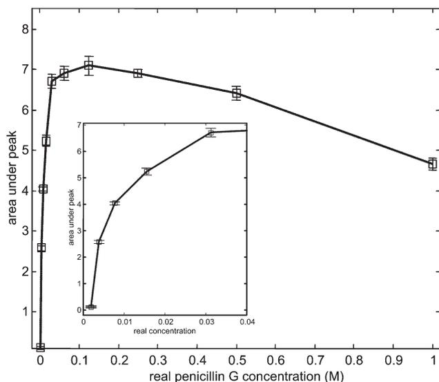
**Fig. 6** Plot of the SERS peak area under  $1606\text{ cm}^{-1}$  versus the penicillin G concentration. The inset shows quantification at low concentrations of penicillin using SERS, whereas at the higher concentrations peak areas appear to decline. Data plotted as means with standard deviation error bars.
