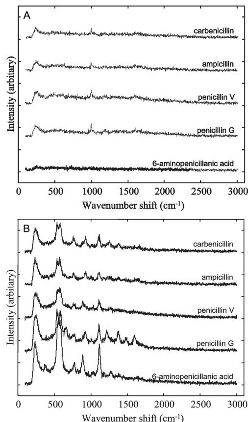
**Fig. 2** (A) Raman and (B) SERS spectra of the five different penicillin molecules (all at 62.5 mM). All spectra were collected for 10 s with a single accumulation. The baselines of the spectra are flattened for illustration purposes only and it should be noted that when carrying out the data analysis no baseline correction was carried out.
