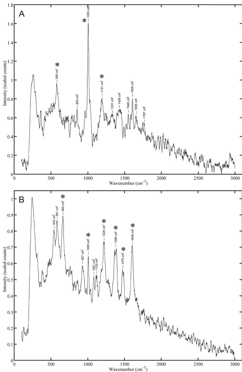
**Fig. 4** (A) Raman (60 s collect) and (B) SERS (10 s collect) spectra of Penicillin G (1 M). Asterisks show peaks which are linear with respect to concentration (see ranges and details in Tables 1 and 2).
