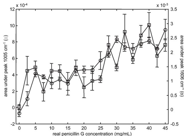
**Fig. 8** Area under SERS peaks from spiked broth (averaged data) smoothed and scaled, plotted versus real concentration of Penicillin G ( $0\text{--}45\text{ mg mL}^{-1}$ ). Quantifiable SERS peaks were detected at  $1005\text{ cm}^{-1}$ , depicted ( $\square$ ), and  $1606\text{ cm}^{-1}$ , depicted ( $\circ$ ). Data plotted as means with standard deviation error bars.
