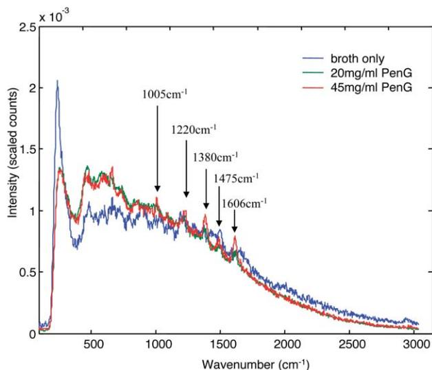
**Fig. 7** *Penicillium chrysogenum* broth spiked with Penicillin G:  $0\text{ mg mL}^{-1}$  (blue line),  $20\text{ mg mL}^{-1}$  (green line) and  $45\text{ mg mL}^{-1}$  (red line).
