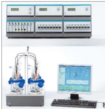
Figure 1. The Dasgip Parallel Bioreactor System with four parallel bioreactors used for culture of CHO cells
